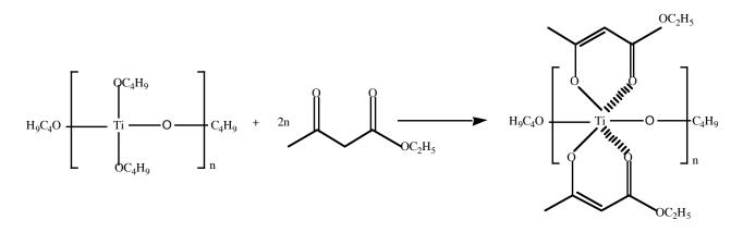
Figure 1. Structure of stabilized polymeric titanium species.
