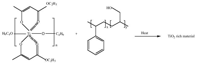
Figure 2. Thermal decomposition scheme of hybrid polymer coating (OptiNDEX A07).
