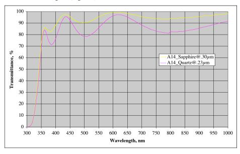
Figure 6. Comparative transmission curves on quartz and sapphire substrates.
