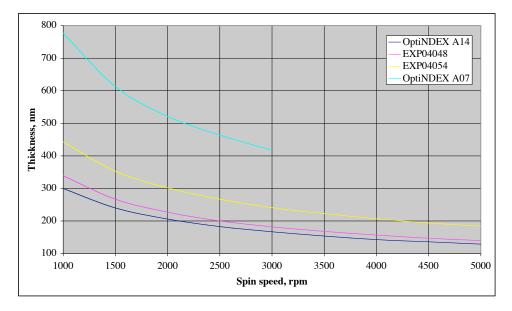
Figure 3. Single-coating film thickness (cured at 300°C for 10 minutes, 225°C/10 minutes for OptiNDEX A07) versus spinning speed.
