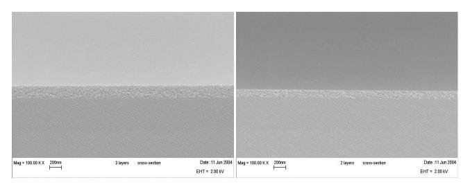
Figure 7. SEM images of two-layer coating (left) and three-layer coating (right).
