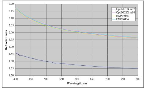
Figure 4. Refractive index spectra of the hybrid polymer coatings.
