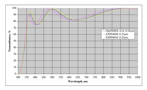
Figure 5. Film transmission curves of the three new hybrid formulations.
