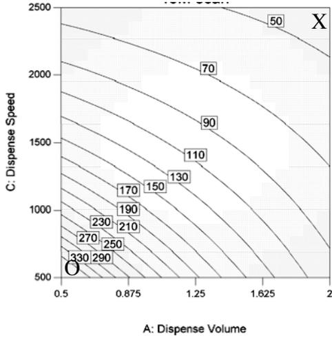
Figure 10. Modeled graph of defects for dispense speed and dispense volume. The “X” denotes confirmation run processes.
