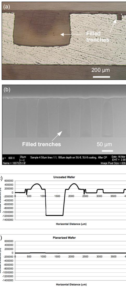
**Figure 4.** Images of filled trenches showing complete fill and planarization: (a) 400 μm deep trench (b) 180 μm deep trench with 50 μm width, (c) profile of wafer with 400 μm deep trench before spin coating, and (d) profile after planarization.
