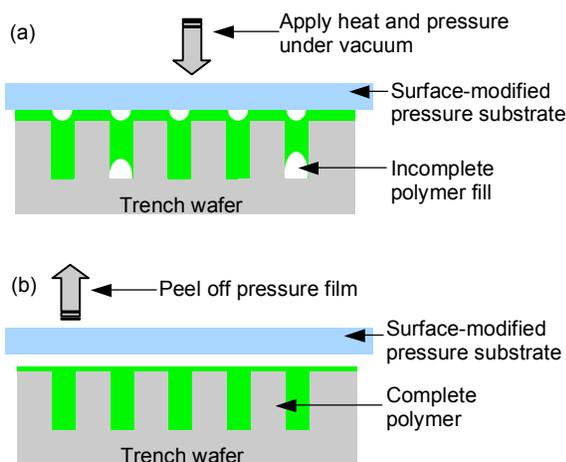
**Figure 3.** Schematic illustration of the contact planarization process
