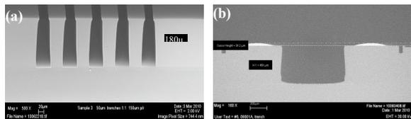
**Figure 1.** SEM image of two test structures created for contact planarization and trench-filling process demonstration: (a) 180  $\mu\text{m}$  deep and 50  $\mu\text{m}$  wide trenches created using thick photoresist on a silicon wafer; (b) 400  $\mu\text{m}$  and 100  $\mu\text{m}$  deep trench in silicon wafer with a 30  $\mu\text{m}$  tall glass frit structure.
