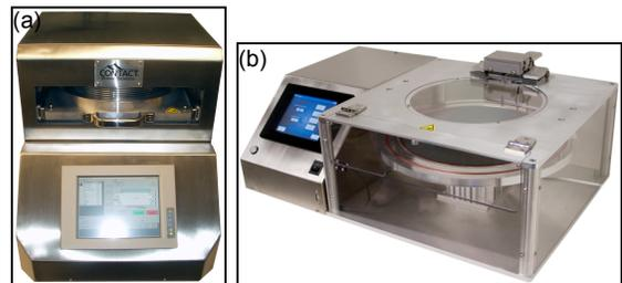
**Figure 5.** Photograph of (a) contact planarization tool and (b) separator tool.
