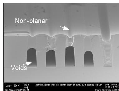
**Figure 2.** SEM image of spin coated trench feature showing the voids and non-planar surface commonly resulting from spin-coating processes for filling deep trenches or vias.
