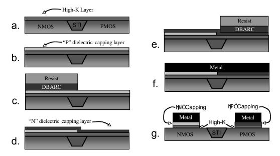
Figure 2: Gate-first HKMG process using DBARC.
