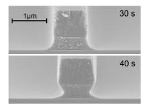
Figure 7: DBARC cross sections through develop time.
