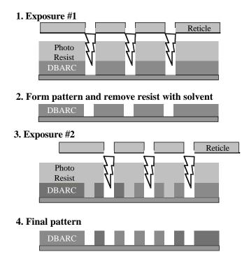
Figure 3: Double-patterning approach using a DBARC.
