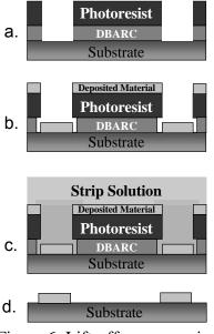
Figure 6: Lift-off process using a DBARC.
