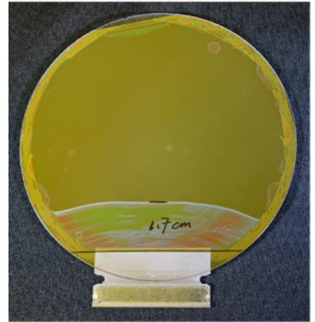
**Figure 6:** Wafer-level Maszara bond strength test.
