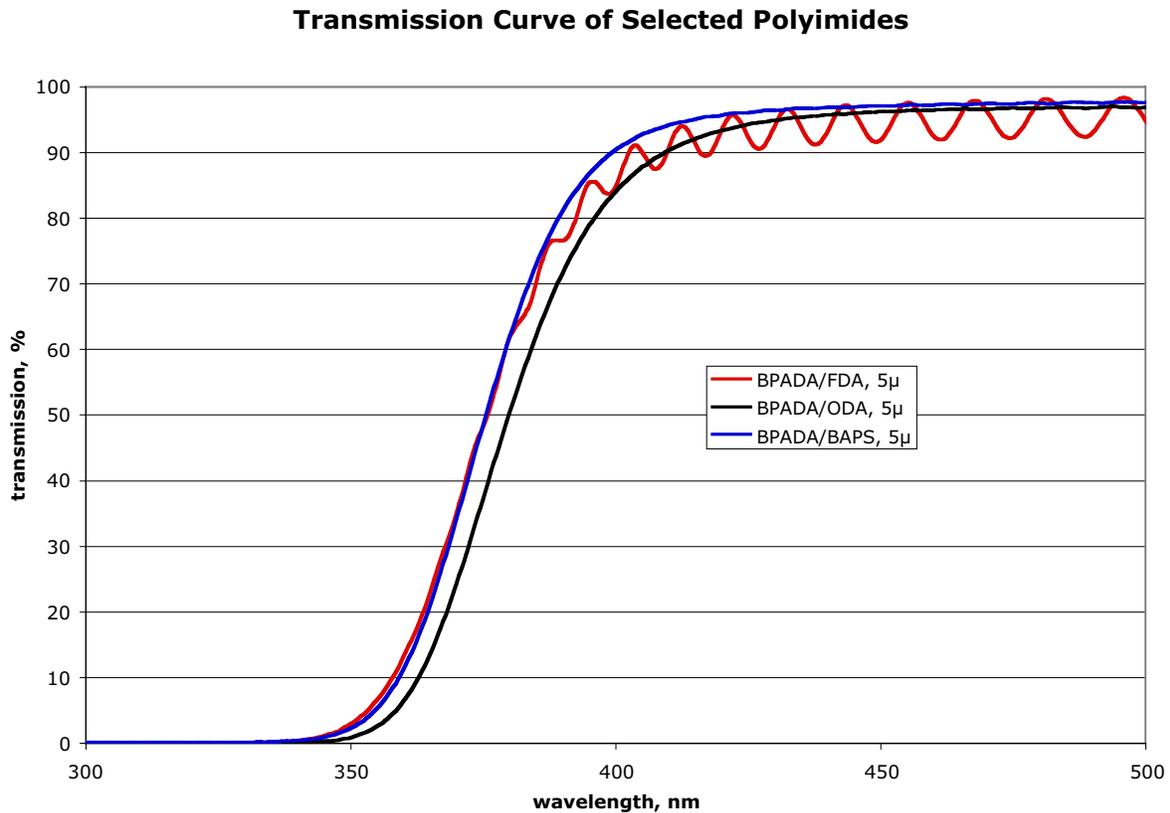
BPADA/BAPS and BPADA/FDA show improved shorter wavelength transmission compared to the reference system. In the case of BPADA/BAPS, this comes at the expense of slightly decreasing the refractive index, but in the case of BPADA/FDA, some improvement in index is observed.
