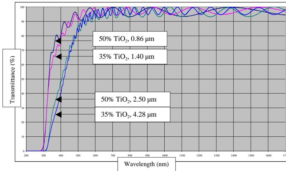
The good optical transparency of the coatings suggested the domain size of the organic and inorganic phases was sufficiently small to not scatter visible light, at least not significantly. A combination of surface plasma etching and SEM examination was used to probe the coating morphology at different metal oxide loadings. The microphotographs
