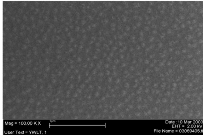
Figure 6. SEM image (100,000X magnification) of plasma-etched surface of high titanium dioxide content hybrid coating.
