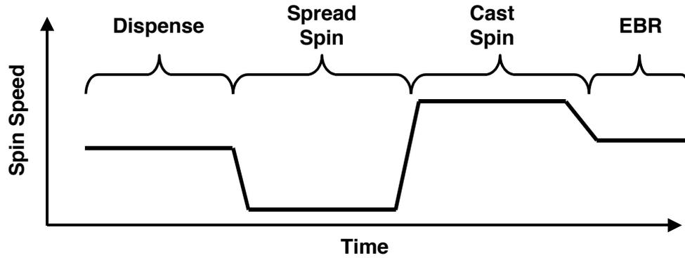
**Figure 1.** Schematic of the new spin process.
