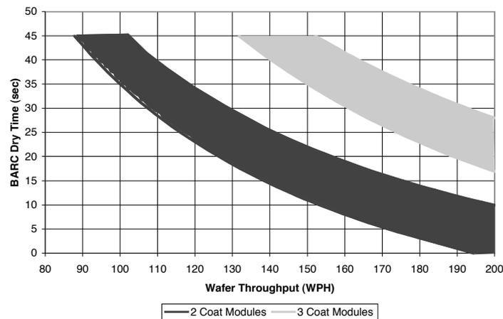
**Figure 2.** Throughput calculation results.
