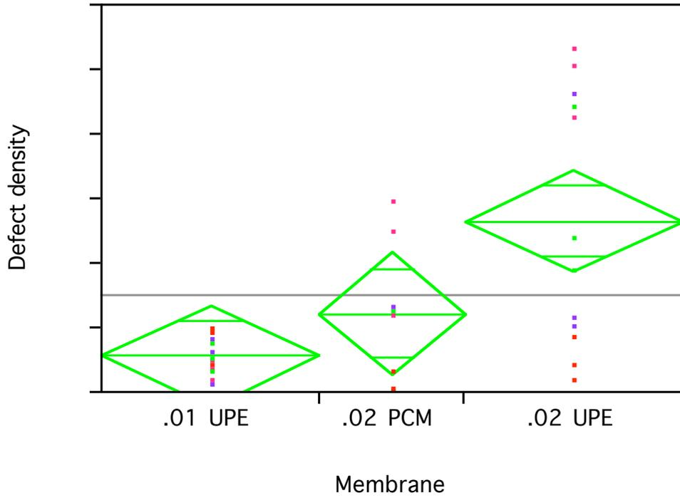
**Figure 3.** Defect density dependence of filter media for DUV112 (includes all filtration rates).
