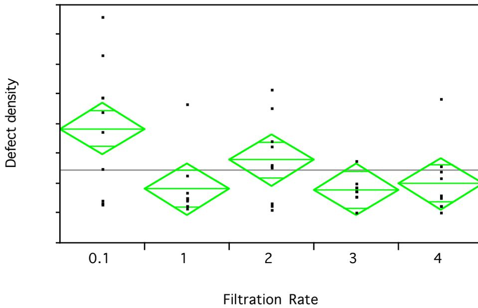
**Figure 4.** Defect density of DUV112 with changing filtration rate (includes all filter media).
