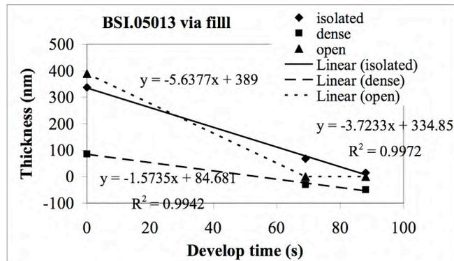
Figure 7. The measurement from SEM cross-section in Figure 6.
