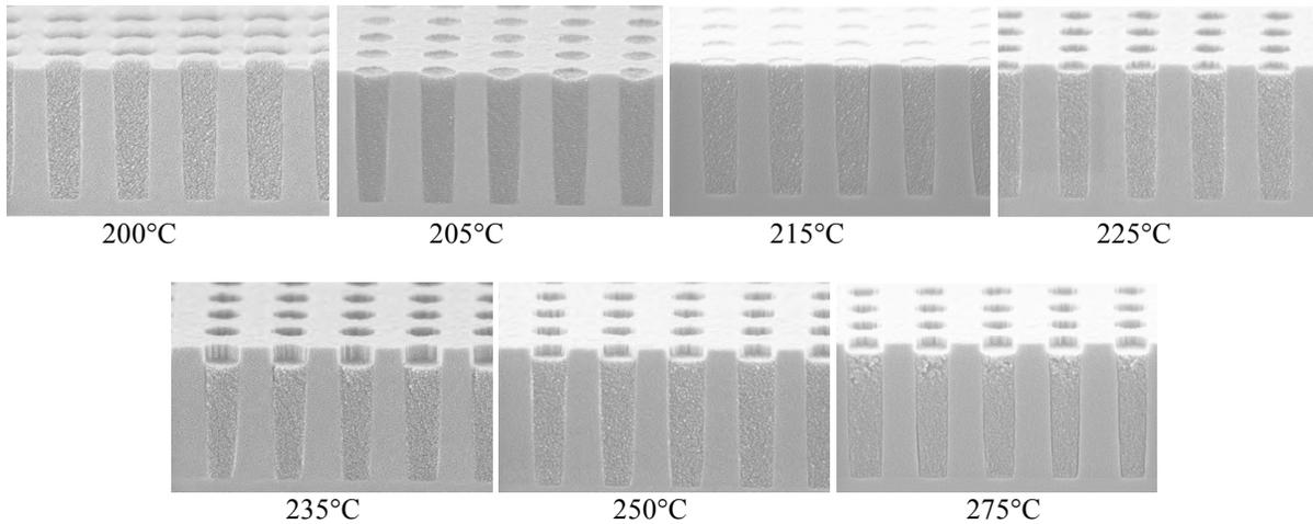
Figure 5. BSI.G05013 is coated on SiO<sub>2</sub> via wafer, and baked at different temperature from 200°C to 275°C. The films are etched back to via top in standard developer.
