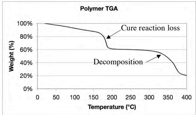
Figure 2. TGA of polymer (temperature ramp 10°C/min in air)
