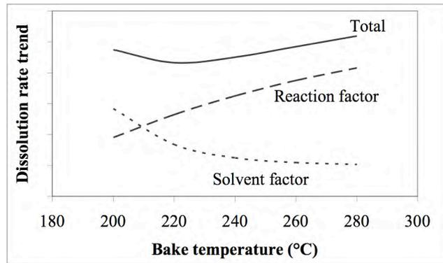
Figure 4. The model of dissolution rate as a function of total of reaction factor and solvent evaporation factor.
