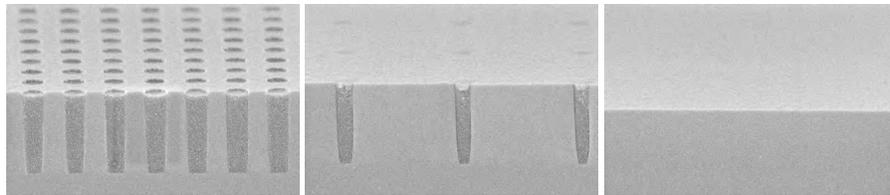
Figure 6. BSI.G05013 SEM cross-section pictures at different areas, dense via (1.5:1), isolated via (5:1), and open, on SiO<sub>2</sub> via wafer. a) no develop, b) develop 69s, c) develop 88s.
