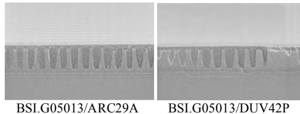
Figure 9. BSI.G05013 applied on  $\text{SiO}_2$  and Black diamond via substrates with different BARCs on the top.
