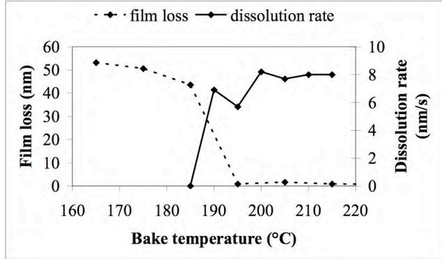
Figure 1. Film thickness loss after PGME/PGMEA mix solvent stripping, and dissolution rate change with bake temperature.
