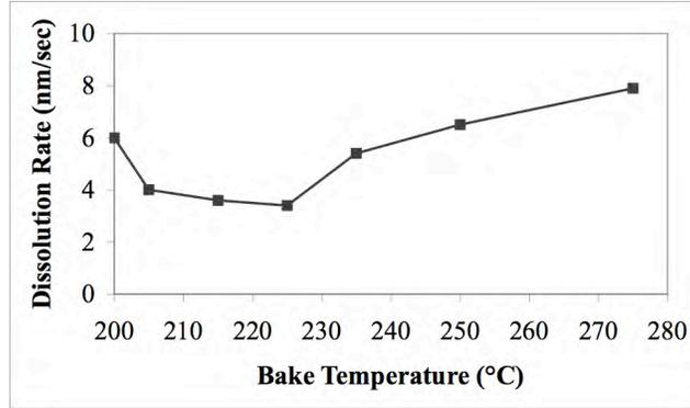
Figure 3. Dissolution rate change with bake temperature.
