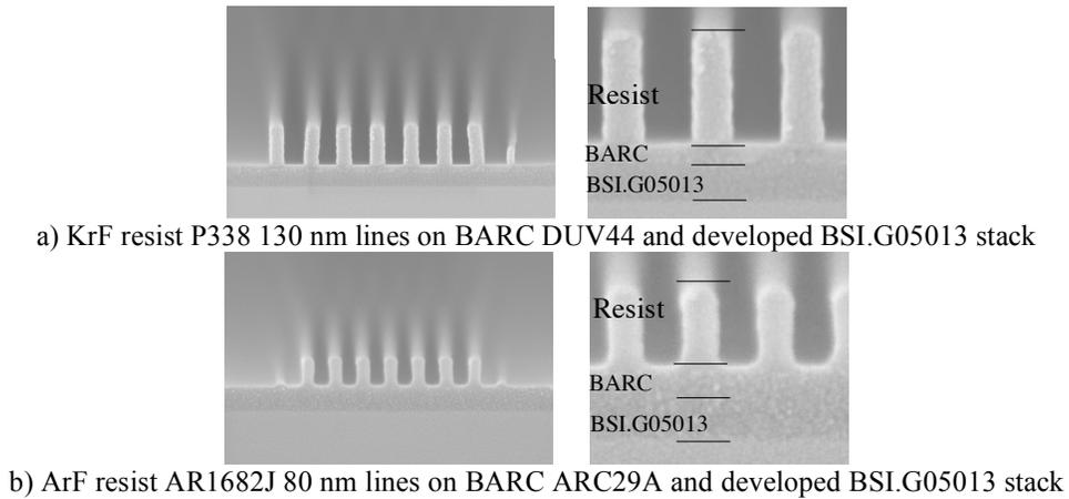
Figure 10. Resist profiles on BARC and developed BSI.G05013 stack, a) KrF lithography, b) ArF lithography.
