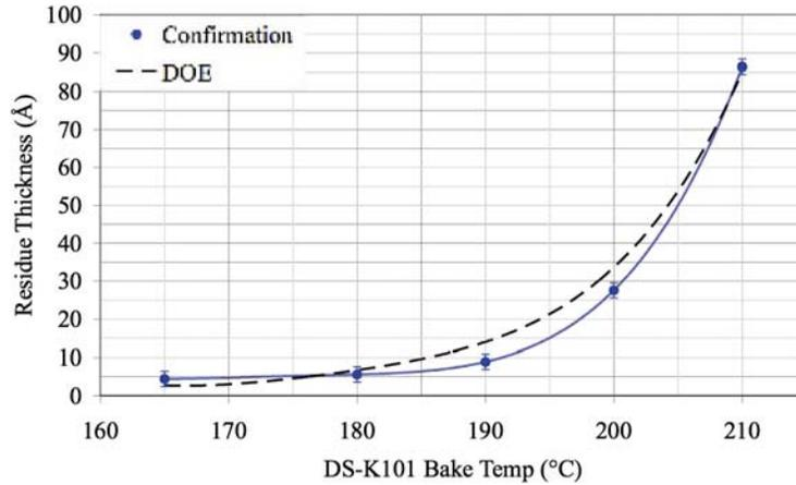
**FIGURE 3.** Bake confirmation of 200-mm track-processed wafers.
