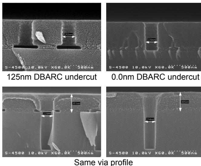
Figure 1: DBARC used in via formation (11).
