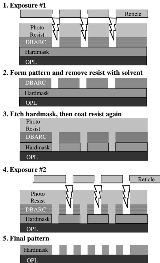
Figure 4: Double-patterning approach using a DBARC and hardmask.
