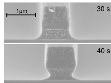
Figure 7: DBARC cross sections through develop time.
