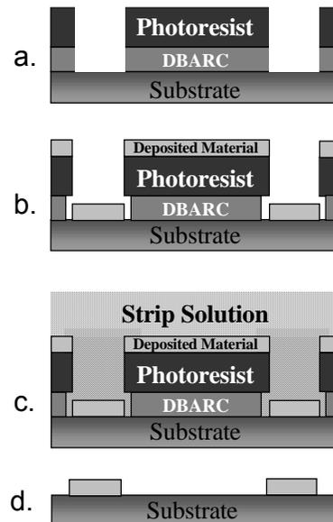
Figure 6: Lift-off process using a DBARC.
