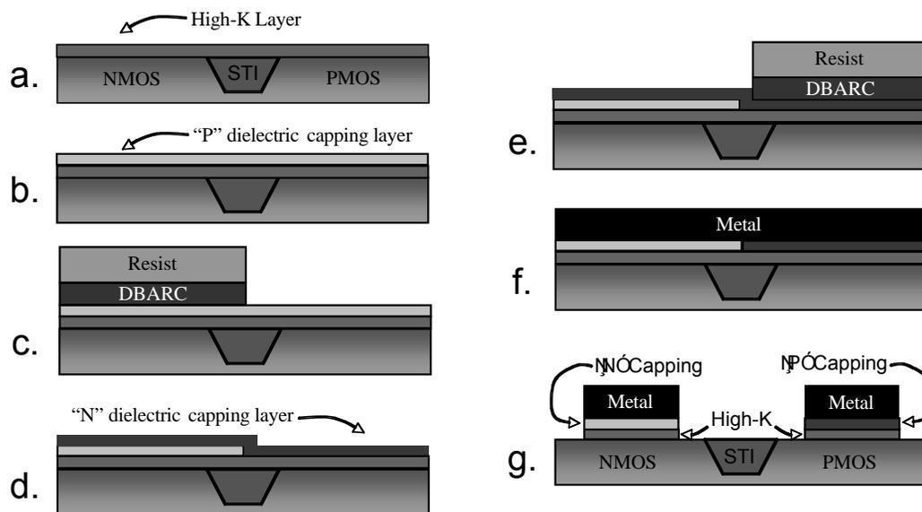
Figure 2: Gate-first HKMG process using DBARC.
