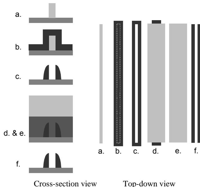
a. Photoresist line. b. CVD layer. c. RIE of CVD layer. d. DBARC and resist pattern. e. RIE of exposed spacer. f. Trimmed spacer after resist and DBARC removal.
