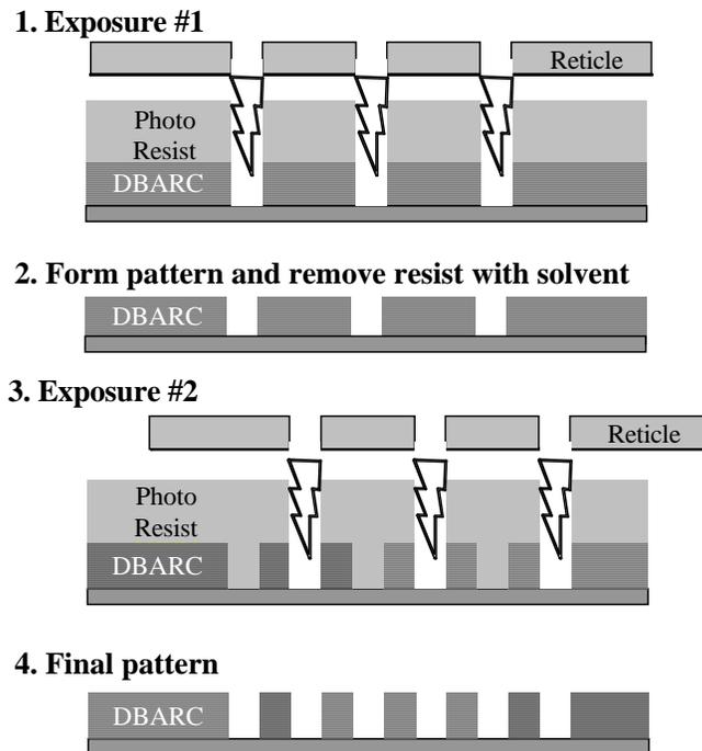
Figure 3: Double-patterning approach using a DBARC.
