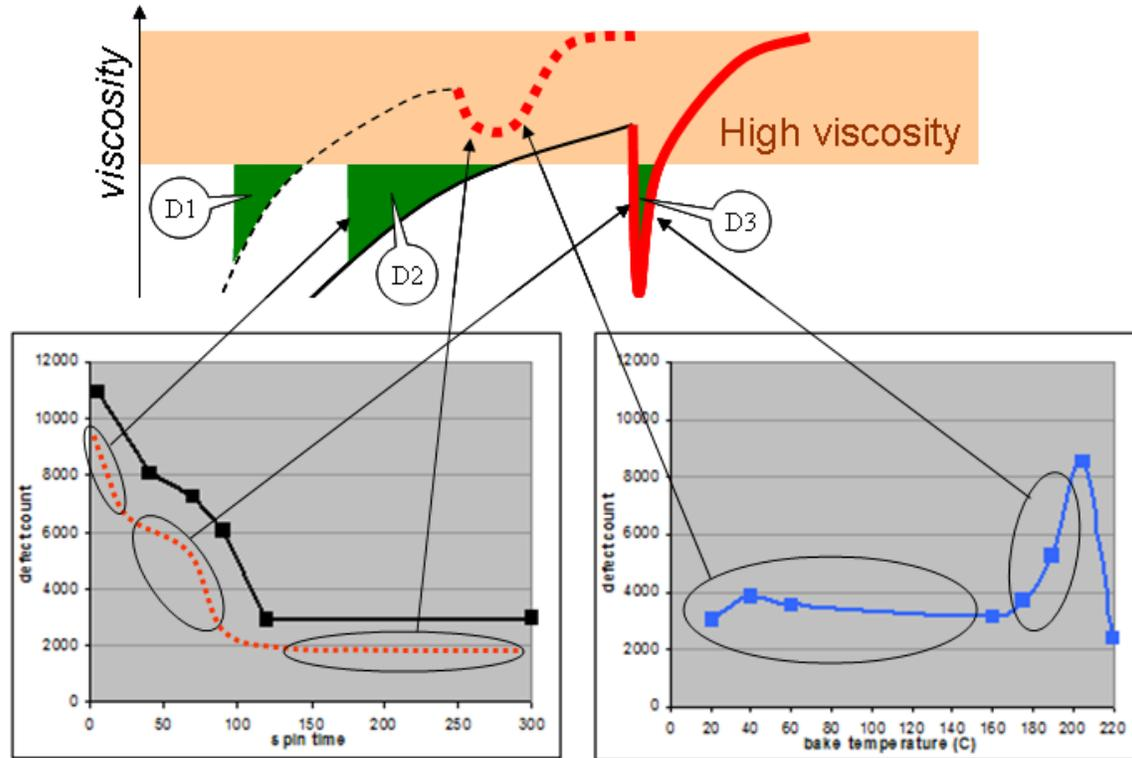
**Figure 2.** Defect count plots from **Table 1**. Spin time test data (wafers 1~6) are plotted on the left; the red dashed line is a theoretical curve. Bake temperature test data (wafers 7~14) are on the right.
