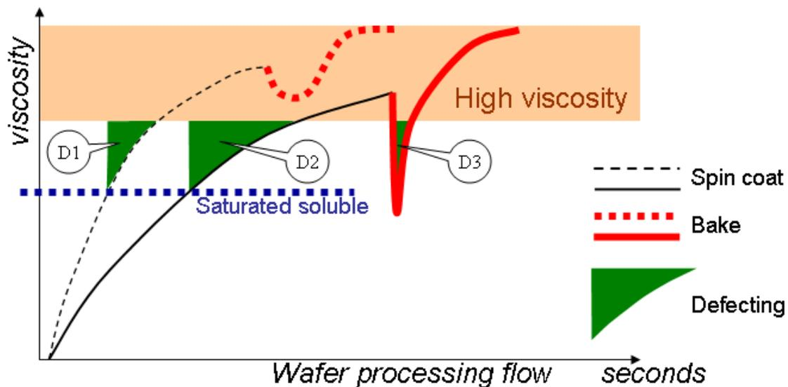
**Figure 1.** Viscosity curve during wafer process flow, where the spin-coating section is represented by the thin black curves and hot plate baking is represented by the thick red curves. The dark green areas indicate the time windows of defect formation. The solid curves represent a conventional a wafer process, and the dashed curves are an improved process proposed for lower defect counts.
