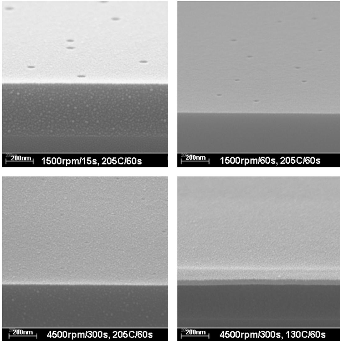
**Figure 4.** Pit defect SEM pictures, with different wafer processing conditions. The drier the material after spinning, and the less reflow upon baking, the smaller the defect size. Pit defects can be completely eliminated when a film is dry enough to prevent reflow.
