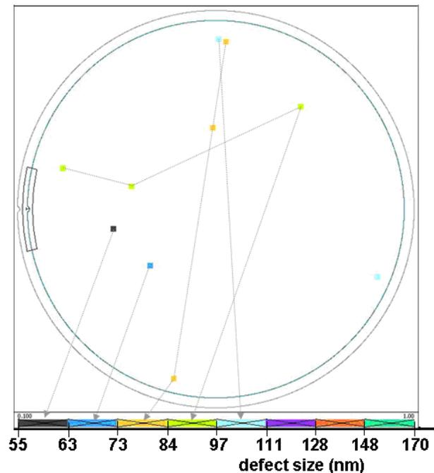
**Figure 4.** Defect map of 8-inch wafer, scanned by SP2 in a class 100 clean room. The coated film is Si-HM material.
