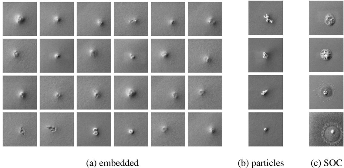
**Figure 3.** Defect patterns of different types from classification: (a) embedded defects from Si-HM – the size is distributed within 70~200 nm; (b) particles considered as foreign defects; (c) larger defects found on SOC coating.
