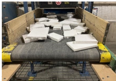
Scrap being fed into the grinding machine
